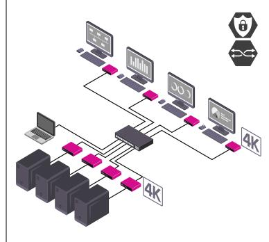
Pathfinder 500 and 800 series endpoints can be integrated into a large matrix system using standard networking switches. Switching between PC's is easily achieved using an On Screen Display (OSD) menu, user definable hot keys or with our intuitive Pathfinder Control software.
