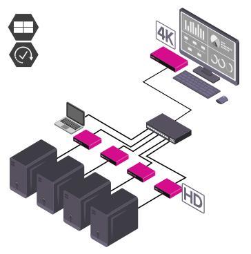
Window**View** allows space saving with easy monitoring and control. Manage up to four PC's from a single 4K monitor; while using only a single keyboard and mouse to control the PC of your choice. Going full screen is simple. One keystroke will make the source you are hovering over fill the 4K screen. If you want to go large, link up to sixteen sources across four displays.
