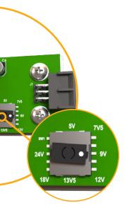
Slide the voltage selector module into the **ONErack Spider.**
