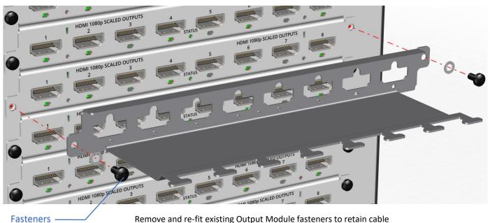
Remove and re-fit existing Output Module fasteners to retain cable retention backet to the desired location.
