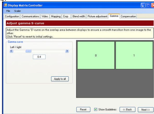
Figure 10 Blend Gamma Curve Adjustment
