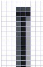
If we take a single line of pixels and look at them closely we will see for a non aliased image solid pixels of one colour .If we look at a line when anti-aliased we can see that no longer is the leg made of solid pixels but of varying shades this will cause an increase in complexity and reduction in compression.
