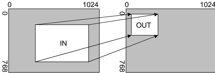
In the example below, 'In' has been set to 300,150 as its top-left source co-ordinate, with a size of 750,400. 'Out' has been set to 50,50 (i.e. close to the top left) with a size of 250,300.
