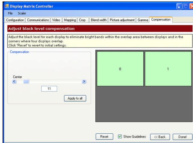
**Figure 11 Black Level Adjustment Screen**
