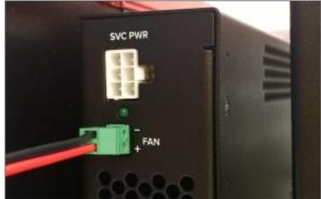
2. Connect the other end of the power cable to the fan cover.
