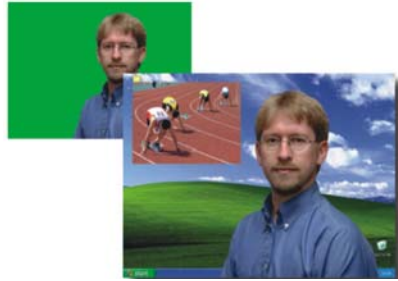
Dual Channel Chromakey with simultaneous P-I-P Insertion
