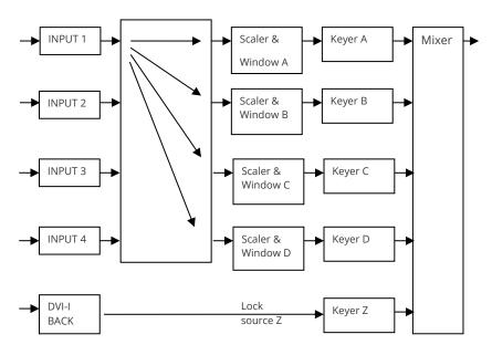
As the diagram shows, the 4 DVI-I inputs are available for use by any of the scalers. A 5<sup>th</sup> DVI-I input acts as a 'lock source' (also known as window Z), which can be used for background / cascading.
