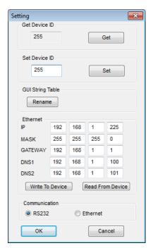
NOTE: After making changes to the Ethernet settings the user must power cycle the unit for the new settings to become effective. If the unit receives commands from both Ethernet and RS-232 ports at the same time the Ethernet commands will have priority.
