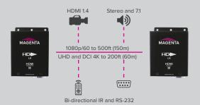
The HD-One DX series is available in HDBaseT and extended range variants in a compact form factor for the transmission of HDMI 1.4 signals including 1080p, 3D, UHD/4K and 4K DCI. Together, the HD-One DX series has full audio support including LPCM 7.1CH, Dolby, TrueHD, Dolby Digital Pluys and DTS-HD.
