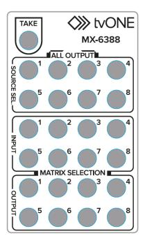
Normal matrix functions are performed by pressing the numbered button of the input you wish to route from the two rows of "INPUT" buttons followed by pressing the numbered button(s) of the desired output(s) from the two rows of "OUTPUT" buttons.
