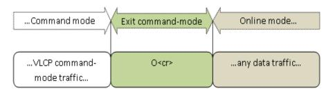
Figure 3. Exiting Command Mode
