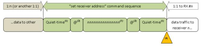
Figure 5. Set Receiver Address Command
