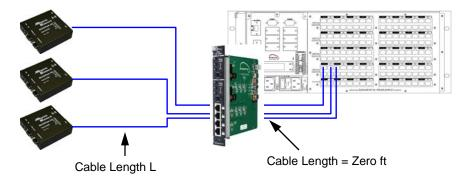
Use the MorphIT Dual EQ card to remove cable lengths from source transmitter just prior to the Mondo III Matrix switch input. Each port on the Dual EQ card can remove 500 ft (152m) of cable length. Two ports may be cascaded to remove a maximum of 800 ft (244m) of cable length.
