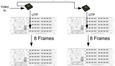
Video out of local monitor port to input of second transmitter
