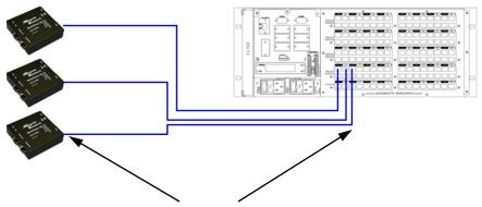
All Cat5 Cable lengths from source Transmitters to the Mondo III Input frame must be within a 30 ft (9m) variance. Add service loops as necessary.
