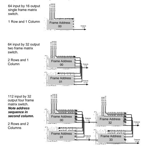
**2.2 Design Guidelines, cont.** Use the following table to determine the correct address assignments and Input Output connections for each switch frame. *Note that Mondo III addressing has changed from legacy Mondo systems*. For legacy Mondo frame addressing, refer to previous Mondo Matrix user guides.
