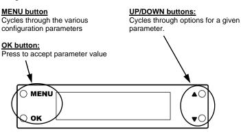
**1. Default / Status** – Displays the firmware version on line one (top) and the Frame Address and Operational Mode on the second line (bottom). This is the "idle" display screen.
