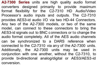
A2-7302 provides an HD-44 interface to 16 AES (8-in/8out) on XLR connectors and a DARS reference input on a BNC connector. This unit contains eight balanced AES to AES3-id converters, plus eight AES3-id to balanced AES converters to provide AES I/O.
