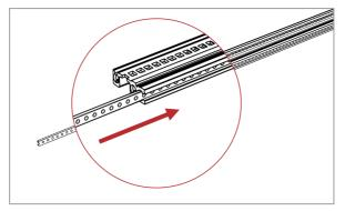
2. Work from the rear of the chassis. Position the lower rail with the numbers facing upwards and the M3 bolt strip facing outwards. Use four M4 screws to connect the rail to the side panels.
